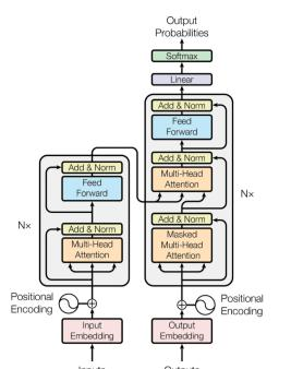
trained Transformer model uses stack of encoders/decoders to process data weighted by attention ouNeed:https://arxiv.org/abs
